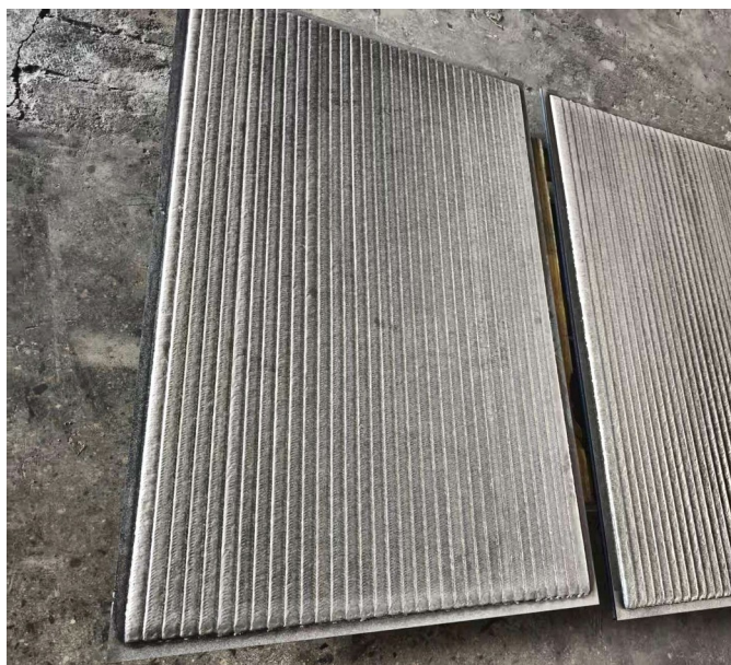
QMAX™ 50 overlay sheets — PTA deposited on mild steel
