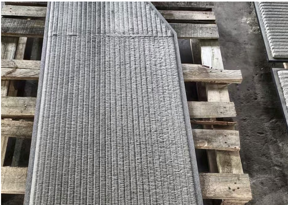
QMAX™ 50 cut panel — ribbed PTA-deposited overlay surface
