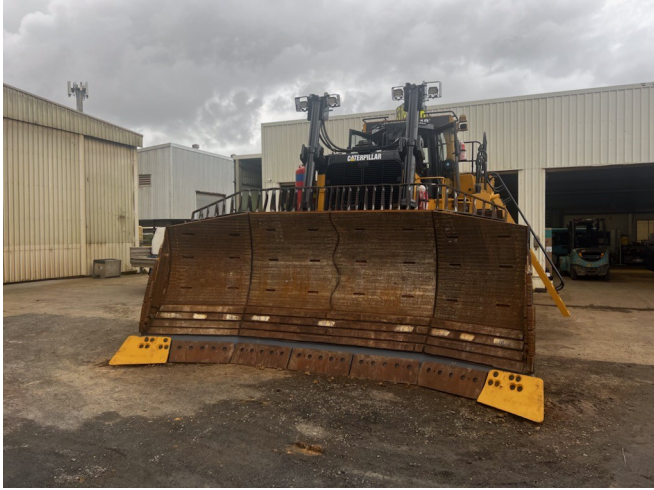
QCLAD™ liner package installed — dozer blade
