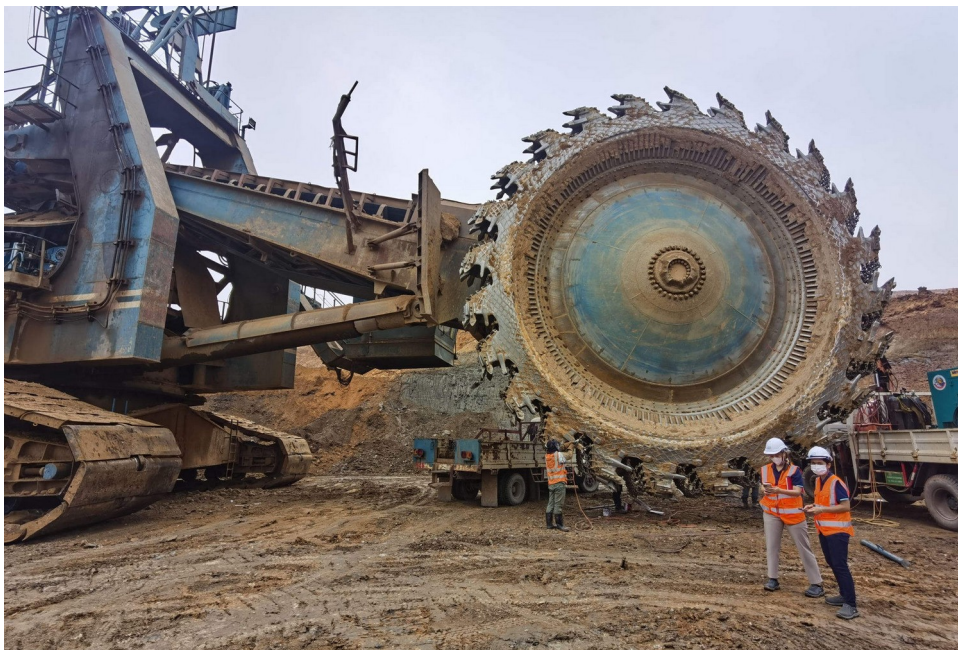
In service — bucket wheel excavator, high sliding abrasion duty
