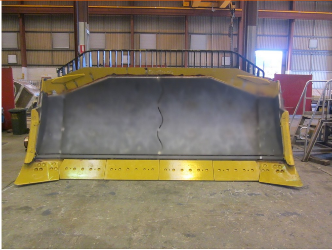
FLOWCLAD™ smooth surface liner installed — dozer blade
